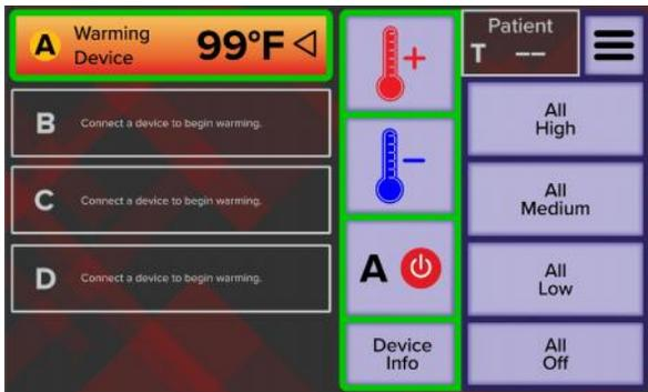
3. The Blanket highlighted in green is the currently selected device. To select Blanket temperature, use the + thermometer to increase the temperature or the – thermometer to decrease the temperature. Turn off highlighted port at the red power icon.
