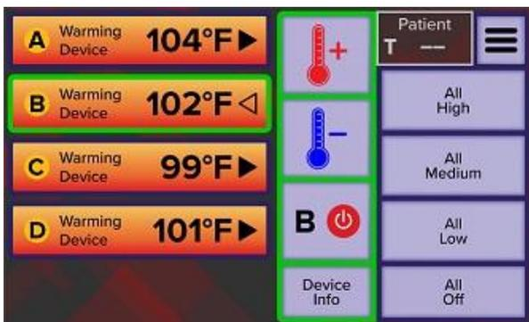
4. Each connected Blanket can be adjusted separately. Other icons to the right adjust all port temperatures simultaneously:
