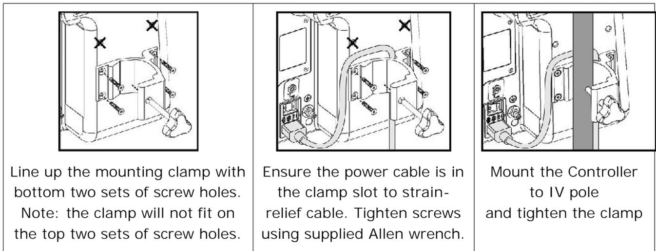
The back of the Controller features a standard VESA 75mm x 75mm interface, allowing for additional mounting options, when using top and bottom holes. The provided IV pole clamp only works with the bottom four holes.
