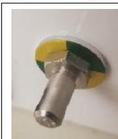
Note: The equipotential stud on the back of the Controller may be used as a grounding point for these tests. Equipotential stud is for ease of attaining ground connection during electrical safety testing. Clip to stud during test. IEC Standard, Reference 60601-1 8.6.7
